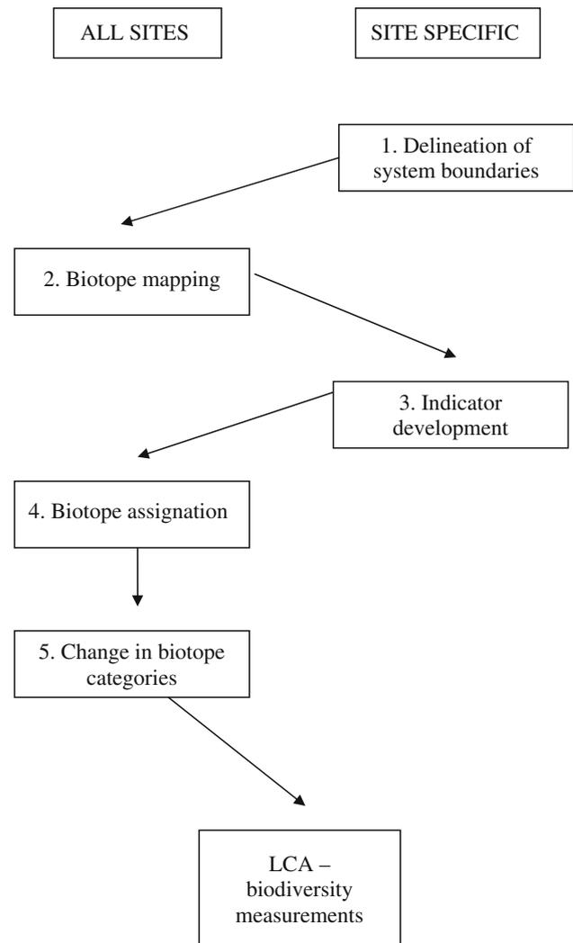
**Fig. 3** The framework of the biotope method showing steps that apply to all sites (left) and steps that require site-specific input (right). In the final step the outcomes of the biotope method can then be incorporated as the biodiversity component in life cycle assessment (LCA)
